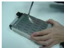
Step 4 Loosen all screws on the Cartridge
