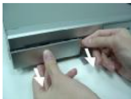
Step 3 Pull out the cartridge
